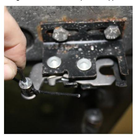
Twist the handle to release the rotary latches and test the door. Make sure both sides latch and release evenly.
